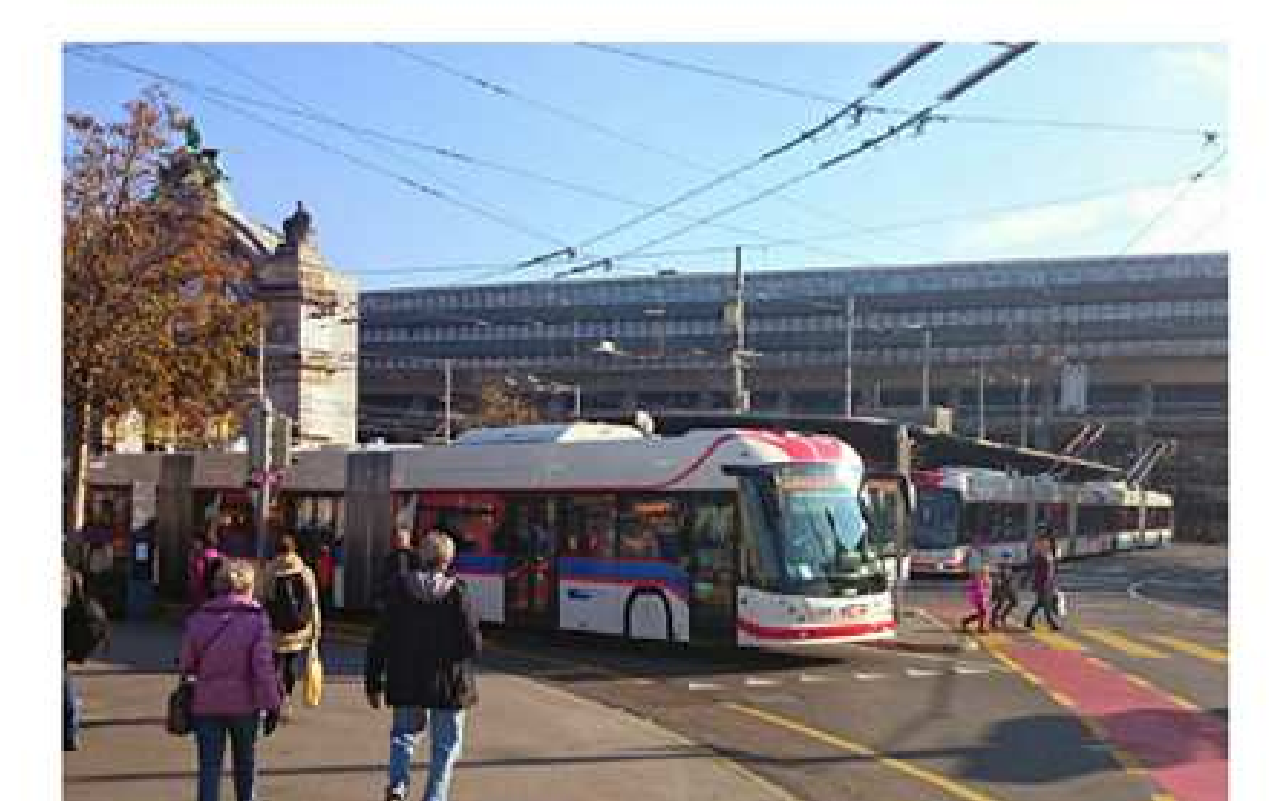
Fig. 1. New 24m HESS trolleybus for 220 passengers (ref. VVL)
