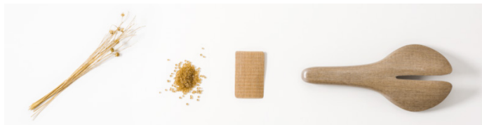
Fig. 5 From flax plants and cellulose based polymers to natural fibre composite parts
