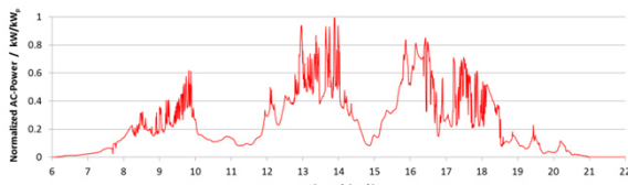
Fig. 1: Normalized power output of an exemplary photovoltaic plant showing strong fluctuations during one day
