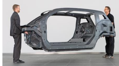
Carbon composite car body of the BMW i3
