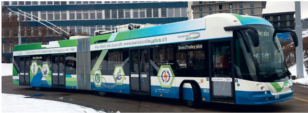
A high-performance battery lets the SwissTrolley plus operate even without a catenary.
