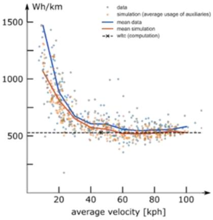
Simulated and measured real-world energy demand as a function of average trip velocity, compared to the norm value obtained in the WLTP. Source: Küng et al.
