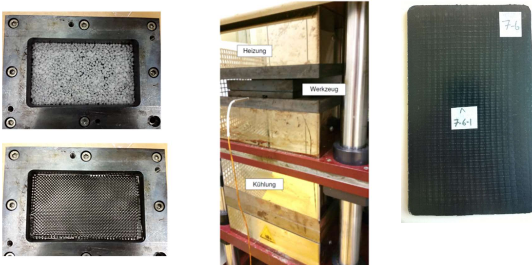
Figure 1.1. Laboratory set-up and obtained plate. Plate dimension 90 x 150 x 3 mm
