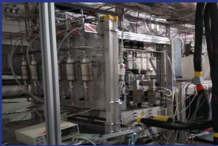
Lab-scale test environment at PSI for fuel cell characterization. The goal is to build a thermoneutral short stack demonstrator (>1 kW).
