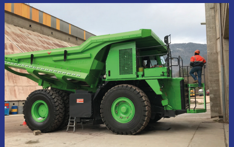
The eDumper (eMining AG) battery cells, -management system and -pack were developed in collaboration with the SCCER Mobility battery research platform.
